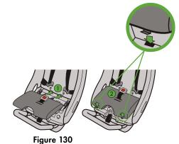
Installing/Removing Anti-Rebound Bar
