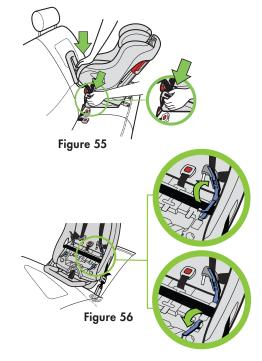
Remove Rear-Facing LATCH Connectors from vehicle lower anchors.
