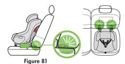
Once the Rigid LATCH Connectors are connected to the LATCH lower anchors, check both LATCH Connector lock indicators located behind the Rigid LATCH Connectors to make sure they have changed from completely red (unlocked) to mostly green (locked) as shown in **Figure 82**.
