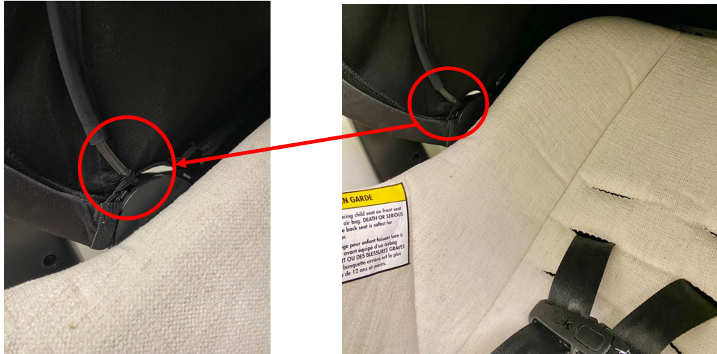
Figures 1 and 2. Location of the canopy stay on the infant car seat
